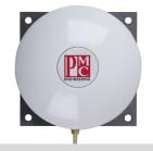
In order to reduce on site maintenance PMC has developed the MP 11 Moisture Protection Reference Volume. For vented gauge transmitters this provides a total isolation to the atmosphere by using a custom bladder while maintaining the high performance of the transmitter. This changes volume with Barometric pressure. Totally maintenance free. Please specify MP 11.
